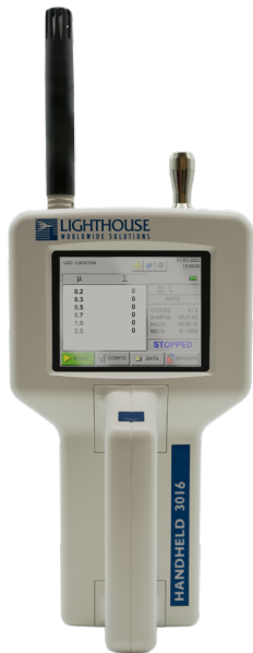
Handheld particle counters – used in remote or some certification applications
