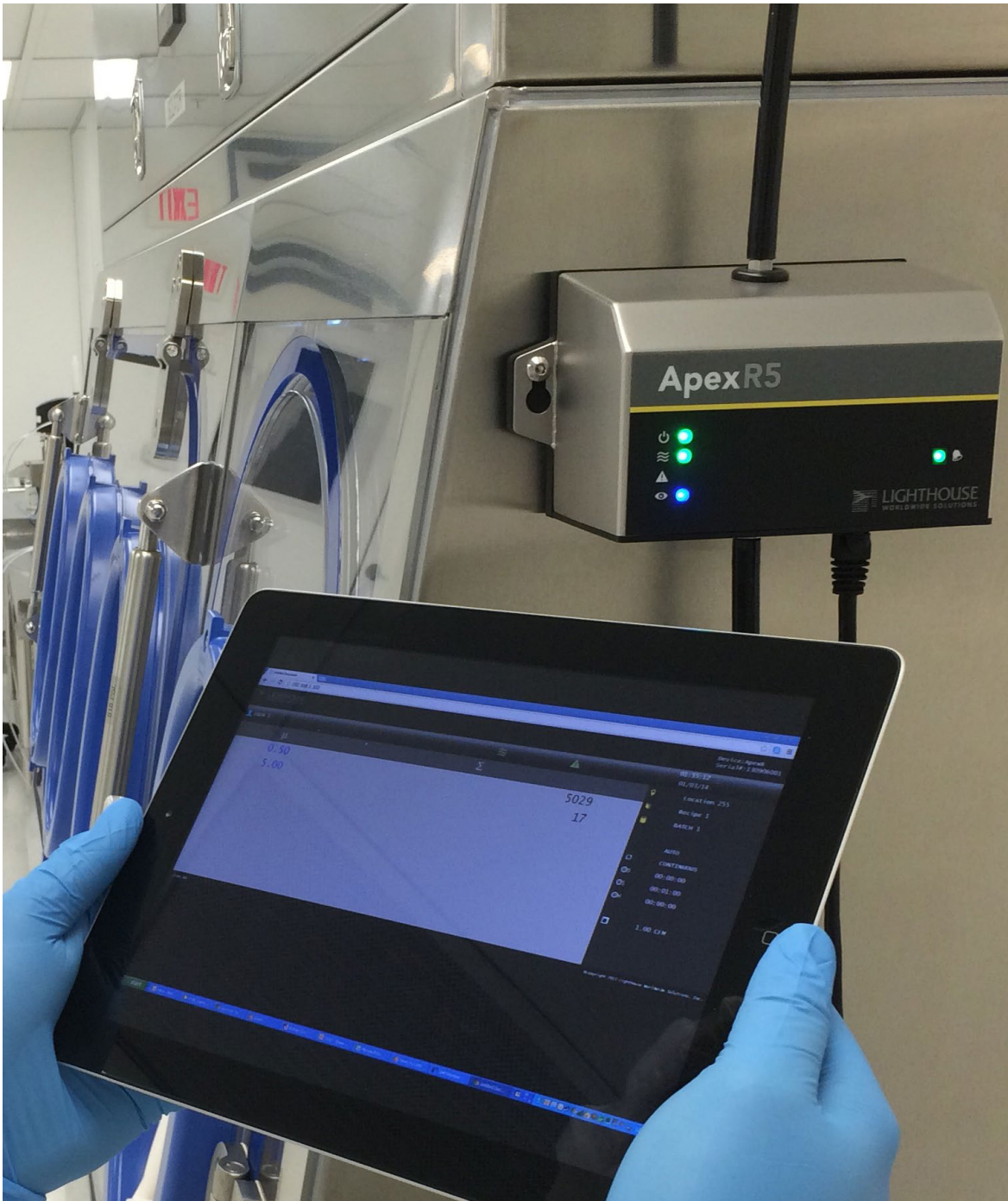
User of EMS system monitoring particle counts in a Cleanroom
