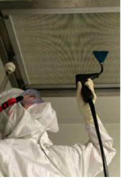
The filter gasket, frame and media are scanned for leaks. The maximum permissible leak is set at 0.01%, although lower limits may be used.
