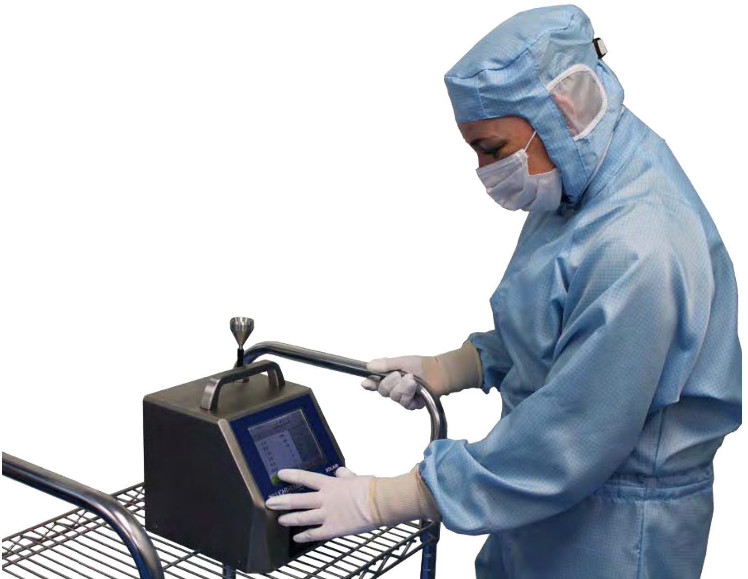
Operator setting up Particle Counter for Cleanroom Certification
