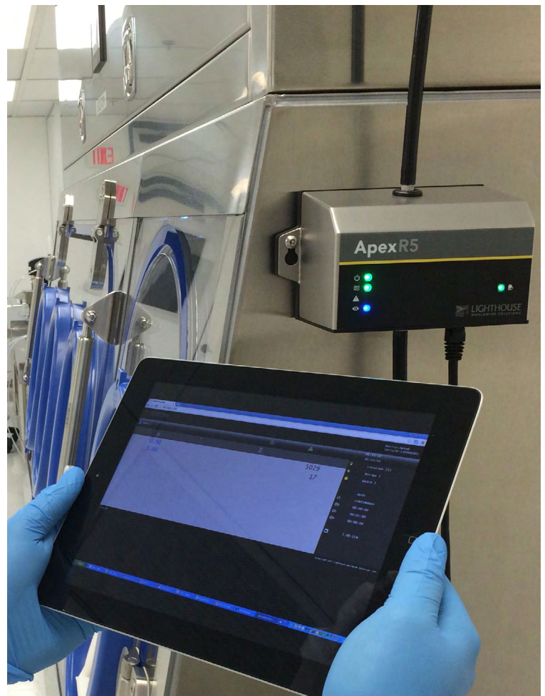
Remote particle sensor continuously monitoring 0.5µm and 5.0µm particle concentrations
