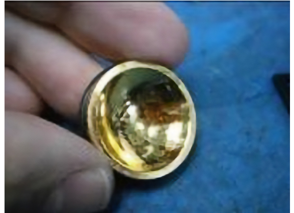
Example of a sensor mirror coated in cleaning solution residue
