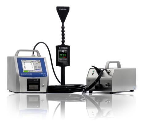
Test equipment used for testing filters includes a particle counter, aerosol generator, dilutor and scanning probe.
