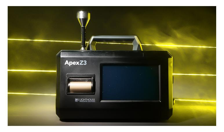
Particle Counters detect, size and count the microscopic particles that we cannot see using a laser, optics, specific airflows and a photodetector. Particle Counters provide visibility in cleanrooms to ensure product quality.
