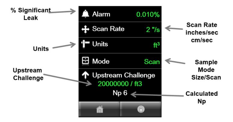
Example of scanning probe test data in real time.
