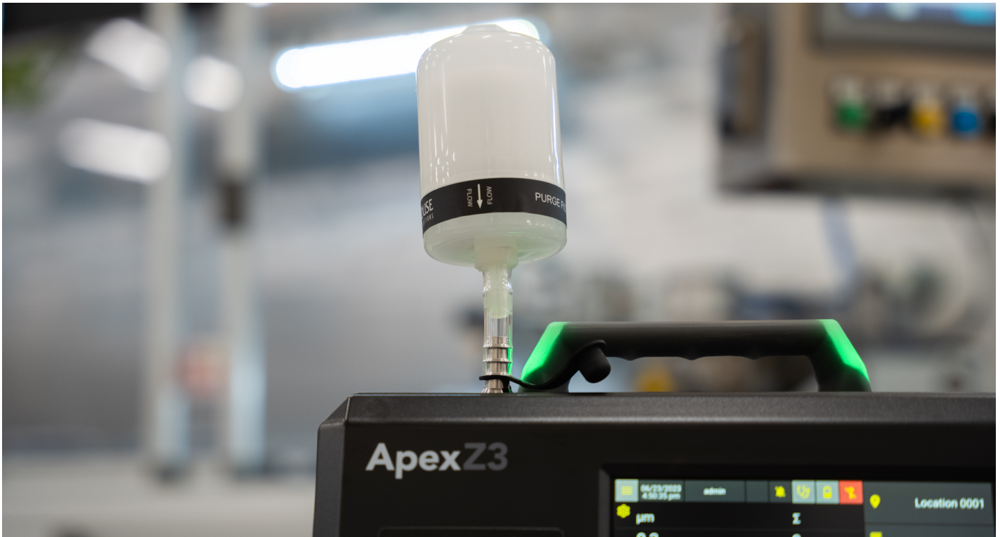
A zero-count filter on an ApexZ particle counter.
