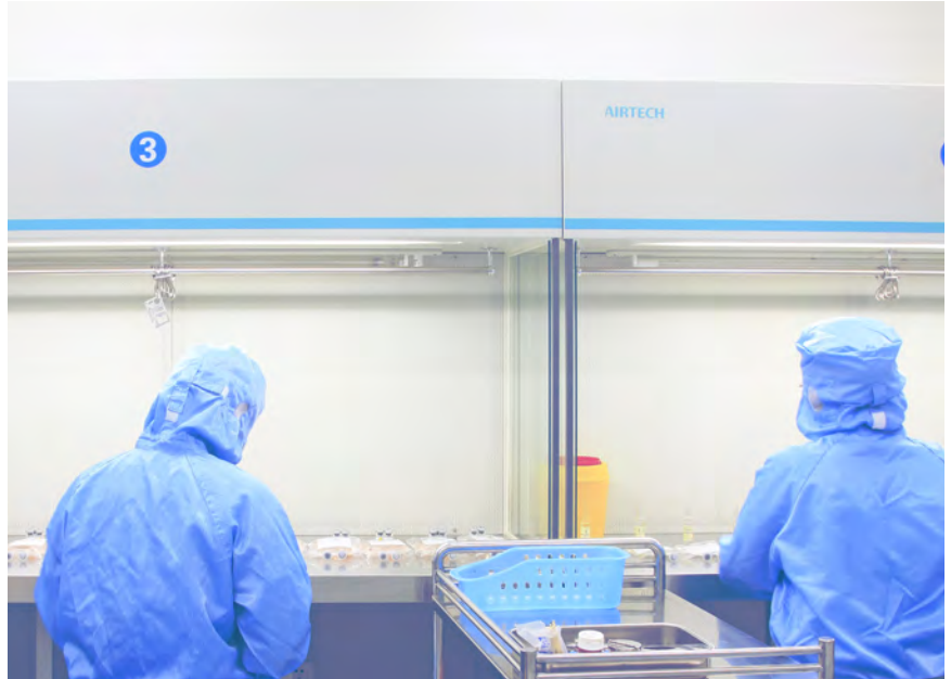
Fig 2.0 Two workers in side by side Laminar Airflow Benches
