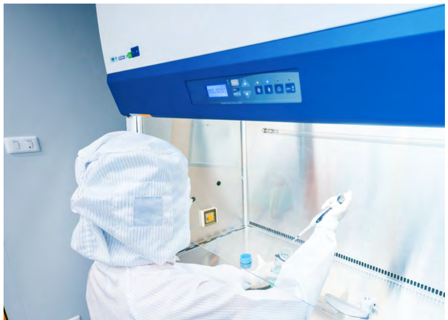
Fig 3.0 Compounding Pharmacy worker working with compounds within a Biological Safety Cabinet.
