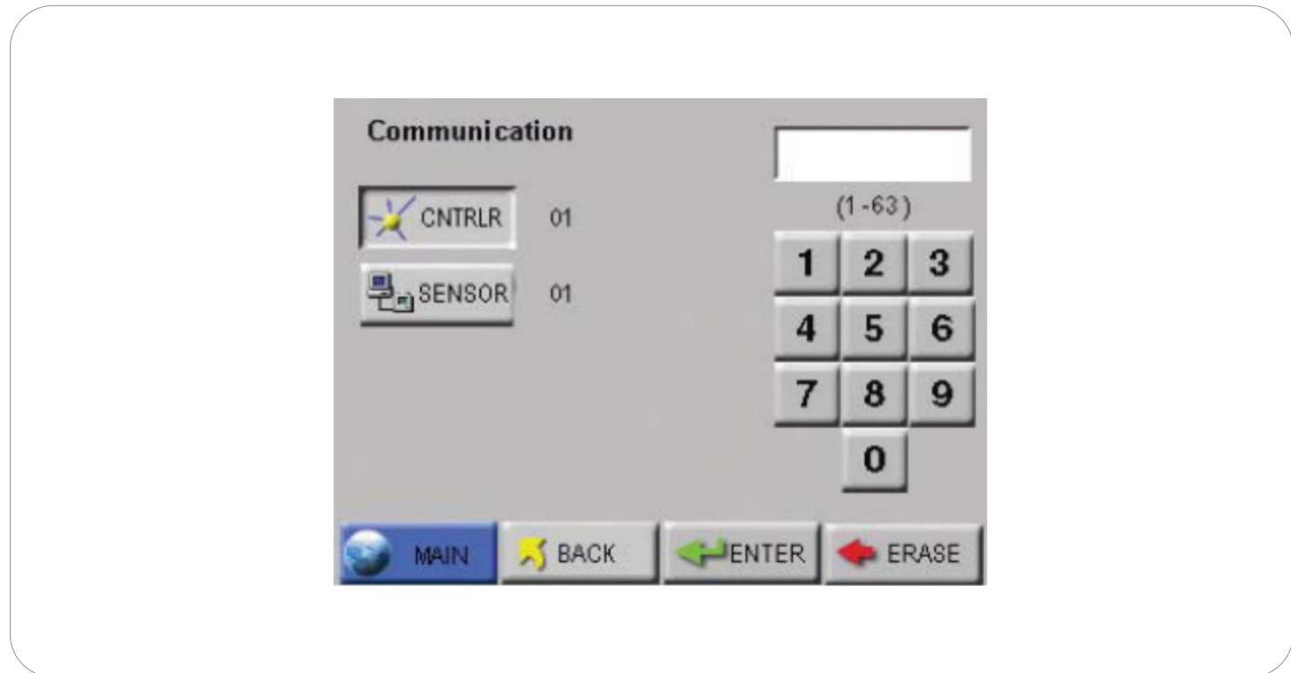
Manifold Controller communication to Particle Counter (Sensor)
