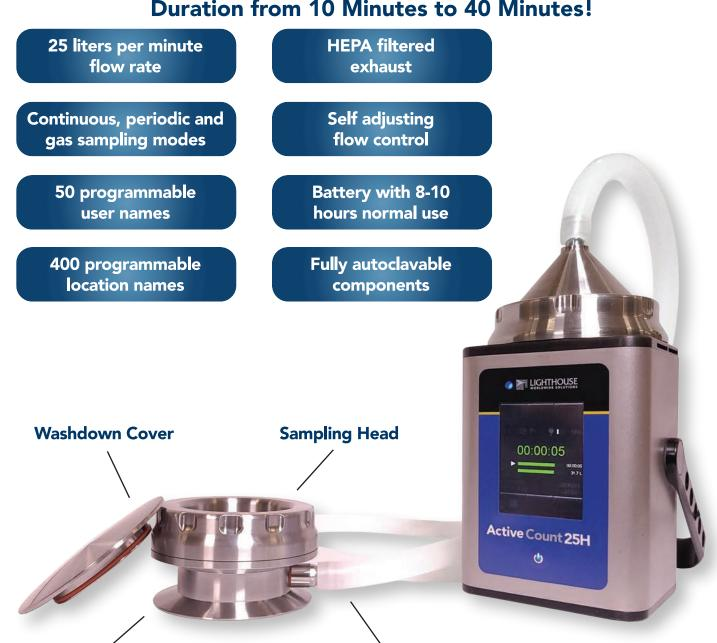
AC25H will allow you to sample 1m<sup>3</sup> of air in 40 minutes, extending your sampling duration while ensuring you the fully compliant with the current industry standards and regulations. This longer duration helps you to lower the number of aseptic manipulations during production while helping you to use fewer agar plates.
