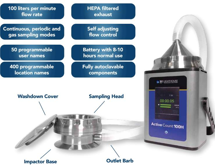
100LPM sampling rate shortened your sampling duration to 10 minutes for a total of  $1m^3$  of air. This reduces the time for cleanroom qualification as well as routine microbiological active air sampling. Periodic sampling mode enables to extension of duration while ensuring full compatibility with the current industry standard and regulations.
