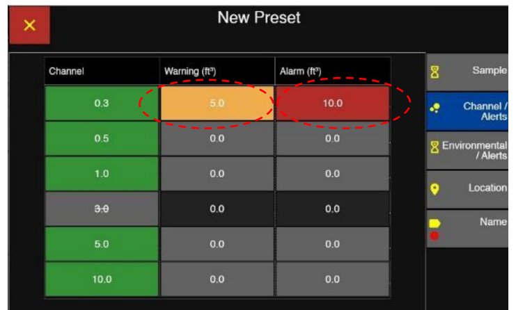
Preset Warning and Alarm settings
