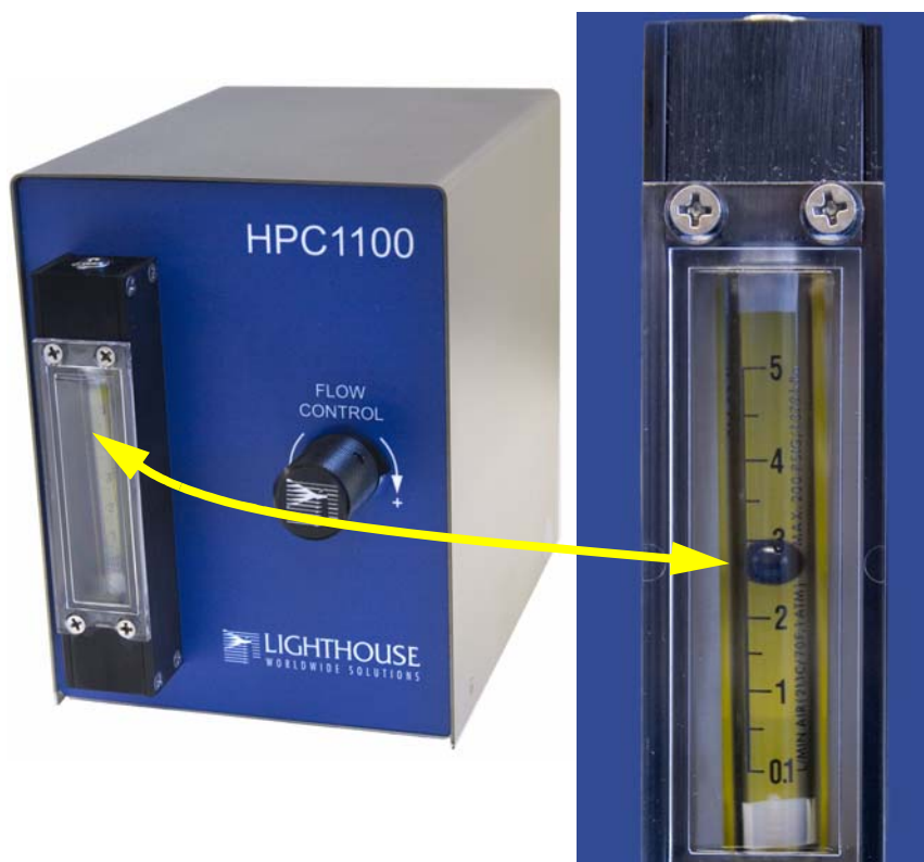
Figure 3-3 Properly Adjusted HPC
