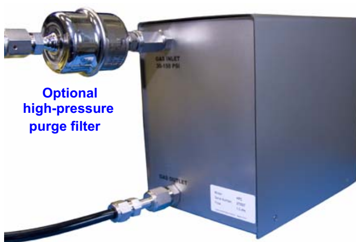
Figure 1-1 HPC1100 with High-Pressure Purge Filter
