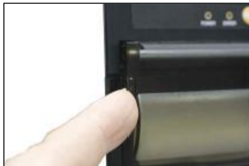
Figure 3-16 Door Latched in properly
