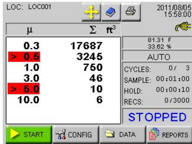
Figure 6-34 Channels in Alarm
