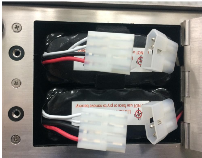
Figure 3-6 Dual-Battery Compartment With Batteries
