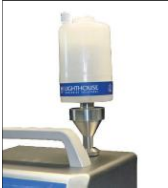
Figure 3-11 ISP Filter Cap Installed
