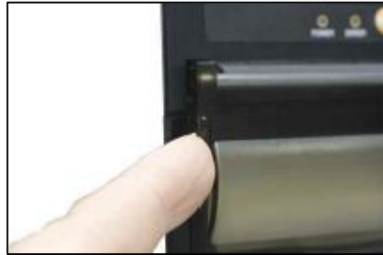
Figure 3-17 Door latched in properly
