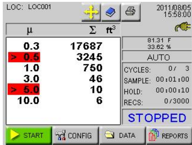
Figure 6-34 Channels in Alarm
