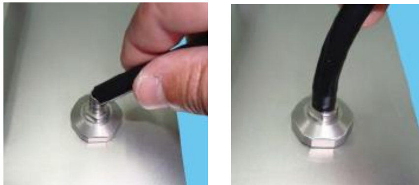
Figure 3-6 Attaching tubing to Inlet
