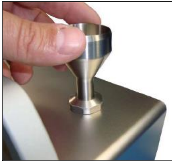
Figure 3-9 Install ISO Probe
