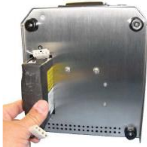
Figure 3-4 Removing the Battery
