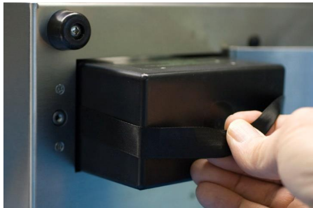
Figure 3-8 Removing Battery (Single-Battery Units)
