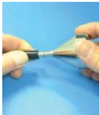
Figure 3-10 Preparing Isokinetic Probe for Use
