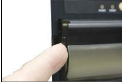
Figure 6-64 Door is Closed and Latched
