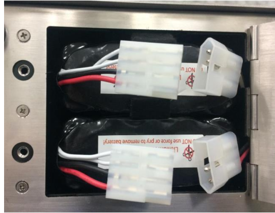
Figure 3-6 Dual-Battery Compartment with Batteries
