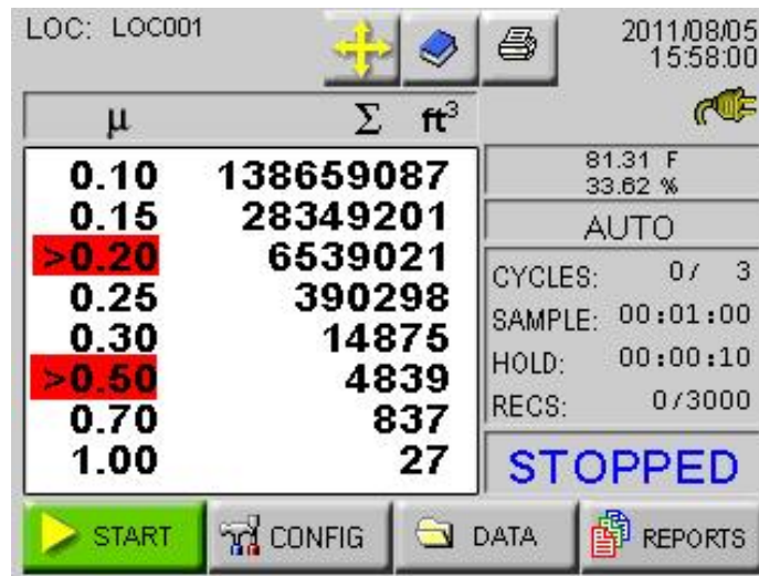
Figure 6-40 Channels in Alarm
