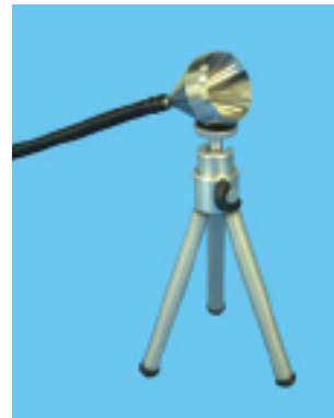
Figure 3-10 Preparing Isokinetic Probe for Use
