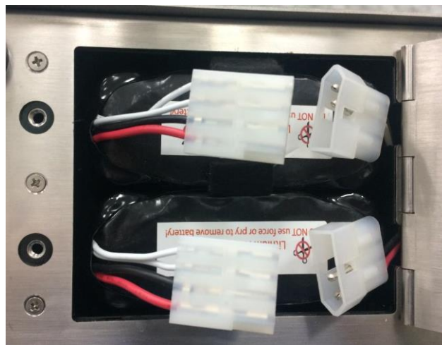
Figure 3-9 Removing Battery (Dual-Battery Units)
