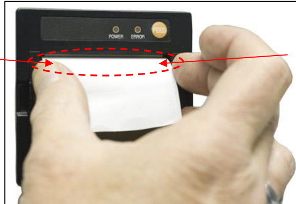
Figure 3-15 Aligning the Paper
