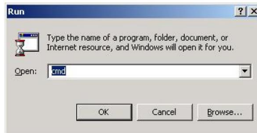
Figure 4-14 Starting the Command Console
