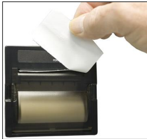
Figure 3-16 Trimming off Extra Paper
