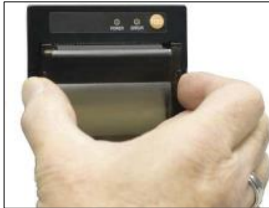
Figure 3-13 Opening Printer Door
