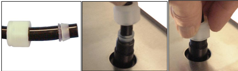
Figure 6-3 Installing Tubing onto Inlet (example)
