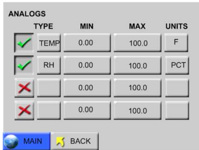
Figure 4-2 Analog Configuration Screen
