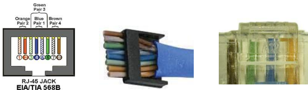
Figure 3-4 EIA/TIA-568B Color Code Example
