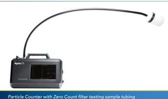
Alternatively, if the application uses VHP sanitation frequently and the tubing is exposed then considerations should be given to the use of 316L Stainless Steel for transportation of particles to the particle counter instead of Bev-A-Line XX.
