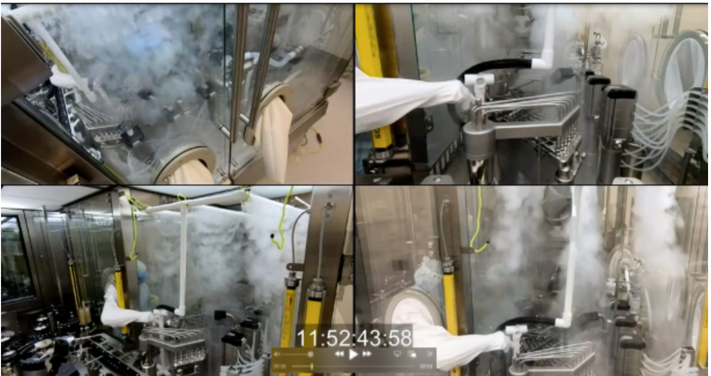
Testing fill head on sterile injectable filling machine
