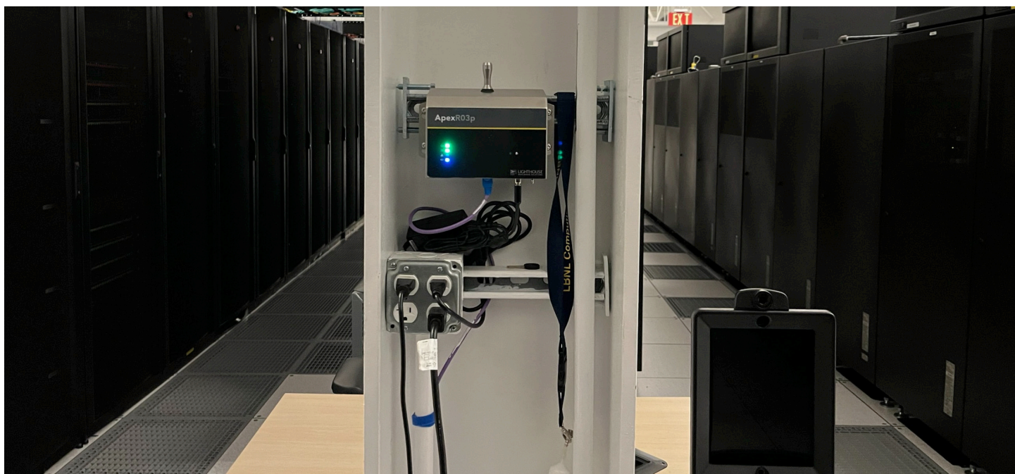
ApexRp Airborne Particle Counter with internal pump installed in the NERSC data center.
